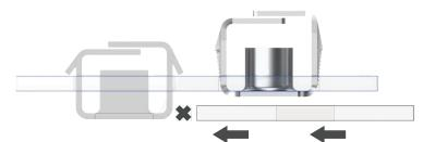
Remains flush and aligned when installed in inverted applications, minimizing transport damage and aiding in assembly
